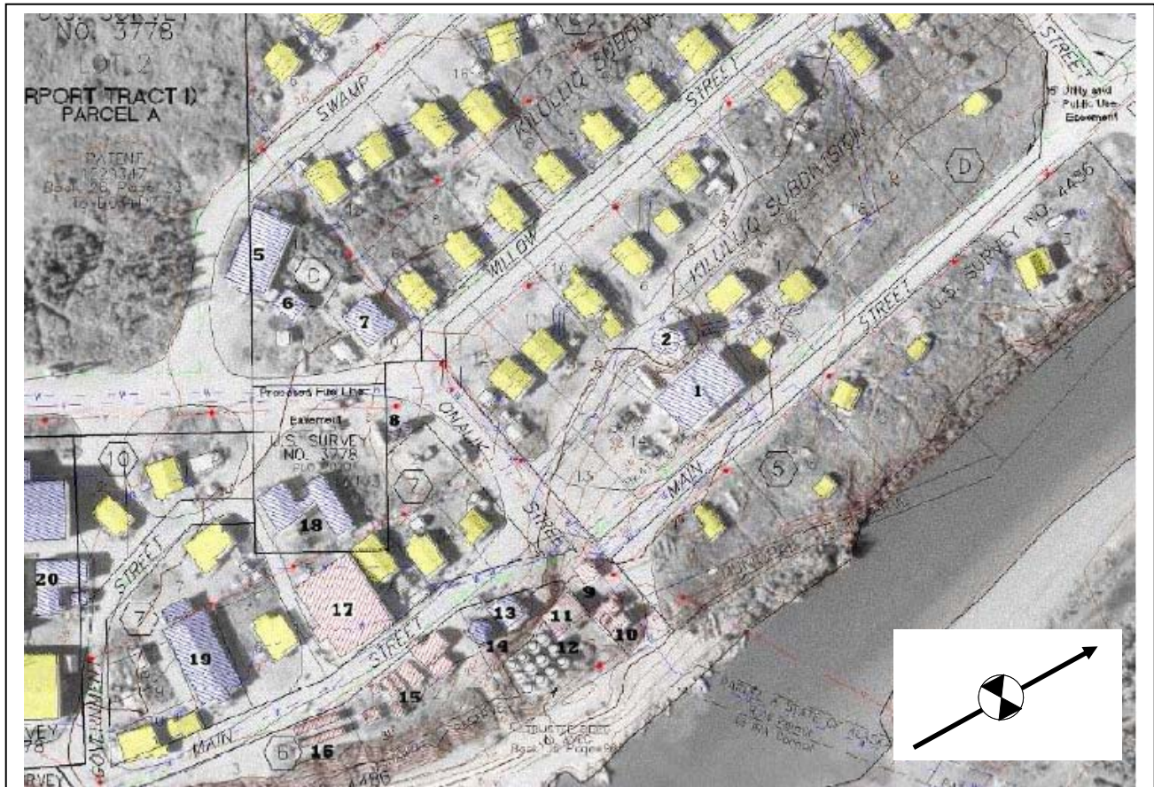
Figure 1. Water Treatment Plant Location (#1 – Water Treatment Plant; #2 Water Storage Tank; #11- Power Plant & Fuel Tank Farm)
