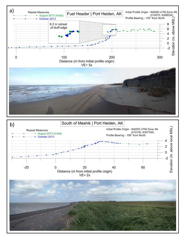
Figure 9. Plots of repeat coastal elevation profiles at the (a) Fuel Header and (b) 'South of Meshik' transects (see fig. 2 for locations). The plot of the Fuel Header transect is accompanied by a photograph taken during the October survey; recent block failures are visible at the toe of the bluff. The plot of the 'South of Meshik' transect is accompanied by a photograph taken during the August survey; this transect is south of the bluffs in a low, dune-backed environment on the southern spit.
